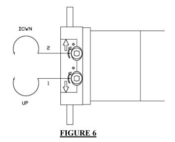
12. The limit switch position is adjusted by turning the screw in clockwise direction to increase the run and in a counter-clockwise direction to reduce the run of the curtain.
