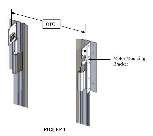
4. The out to out on the track is measured from the back of the mounting plate to the back of the other mounting plate. Locate the track assembly with the motor mount bracket, (See Fig. 1 - Note: Right hand motor mount shown). Mount the track on the OTO mark on the side of the wall where the motor will be mounted. Weld or fasten in place with the proper fasteners, (fasteners not provided).
